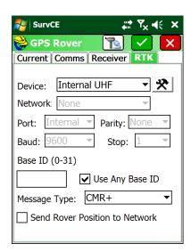
Press 'Hammer/Wrench' to right of Internal UHF:
