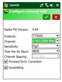
Set as shown for main base, Ch1 is 453.400 which is Utah Hill and Ch2 is 453.250 which is Washington repeater.
